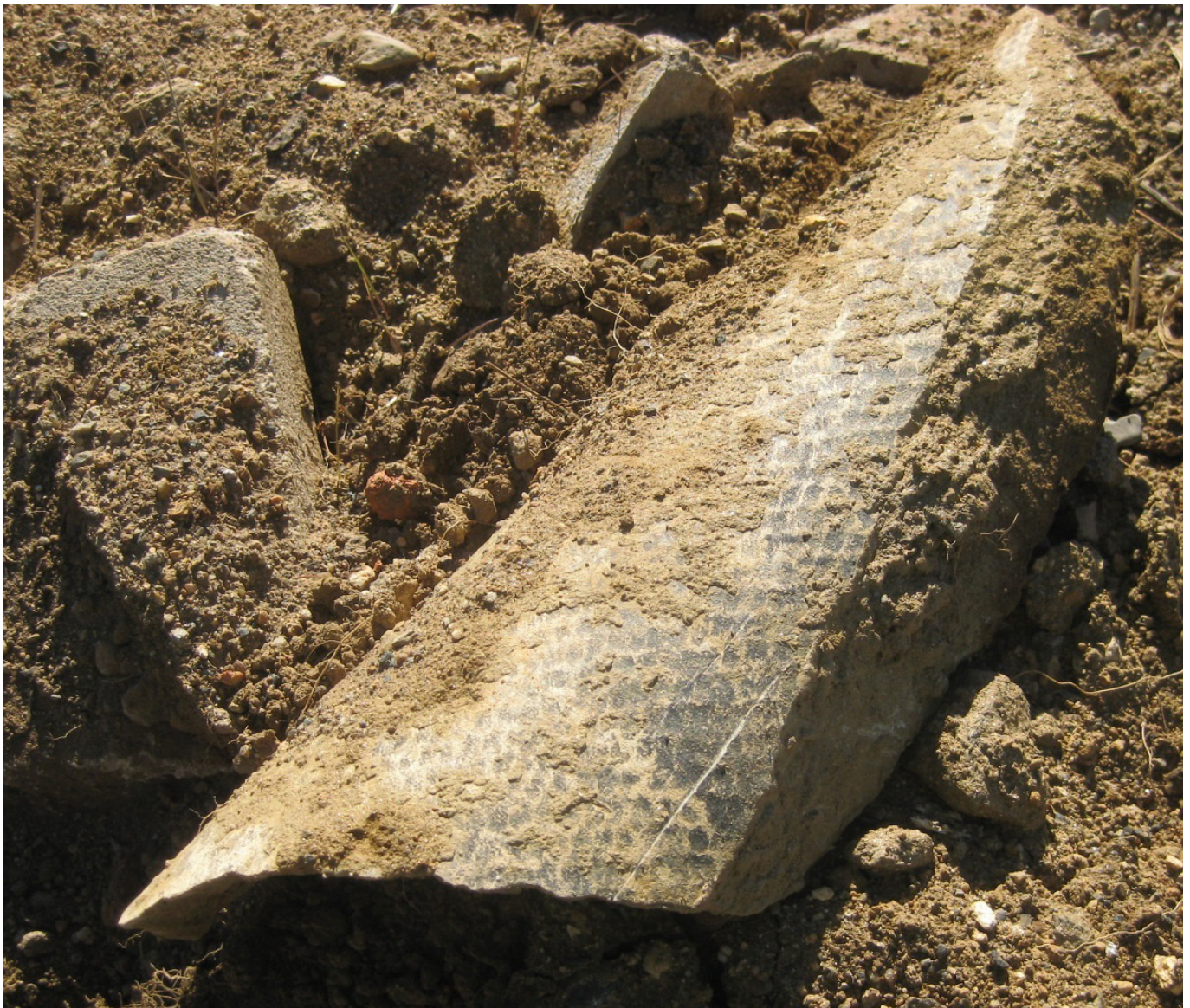
Above: Asbestos pipe
