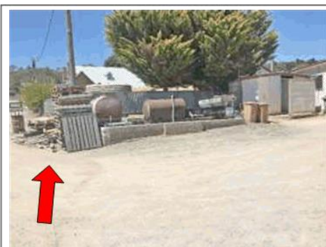
Old pallets used for open fire should represent a trip hazard and fire exposure to the waste oil storage area.
