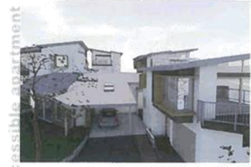
Windyspray® Colorbond steel deck roofing Local granite ledgerstone facing larder wall Local granite ledgerstone facing larder wall Surfmetal® steel corr. wall claddings
