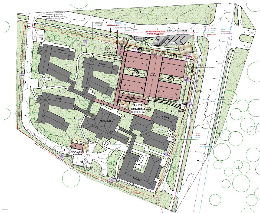
Figure 9 - Layout of existing facility with proposed development in red.
