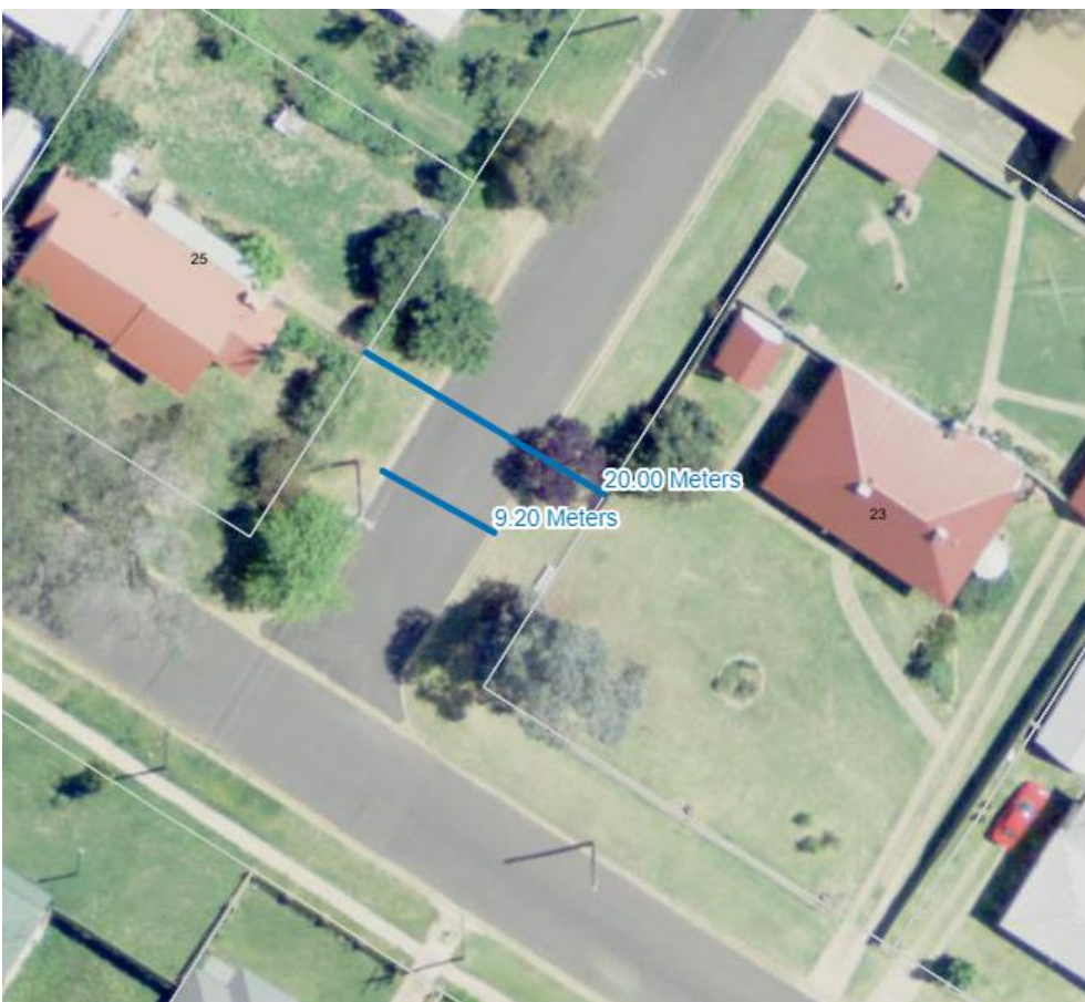
Figure 18: Hoskin Street Carriageway.
