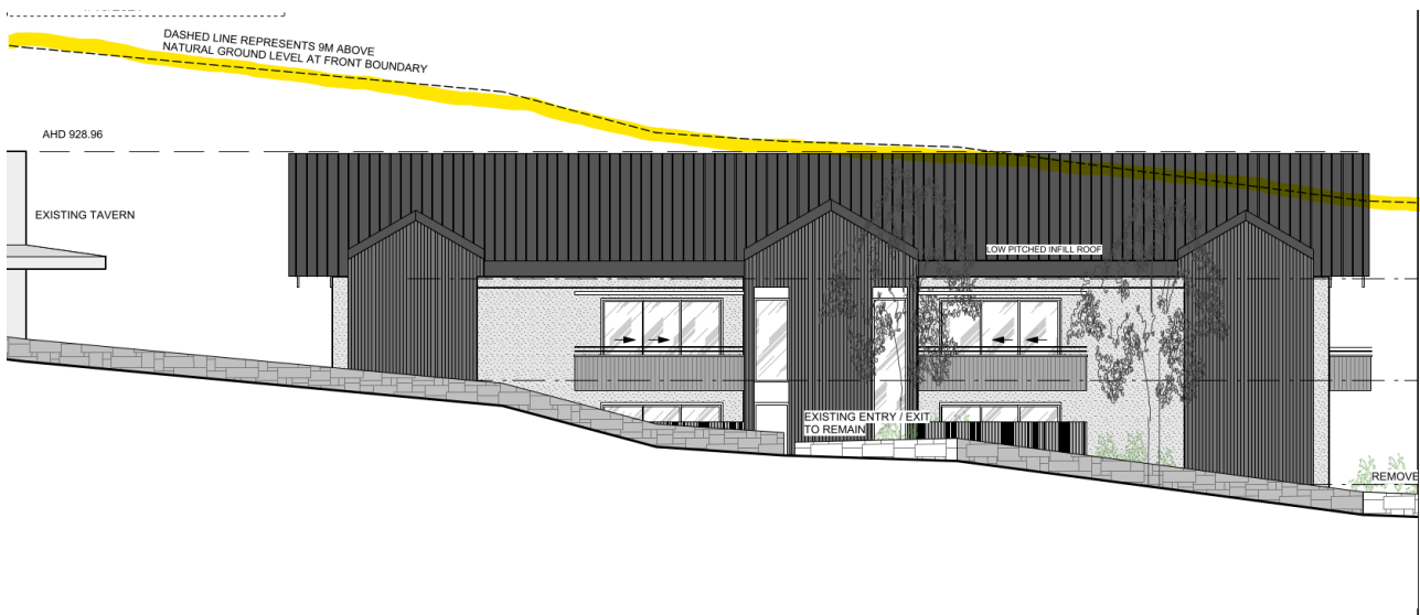
Figure 6 – Extent of height exceedance on the Northern and Western Elevations
