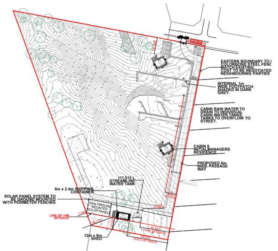
Figure 3: Proposed Site layout – Stage 1 (Cabins 1 & 9 (temporary manager's residence and bushfire refuge), storage shed, solar panels and shipping container)
