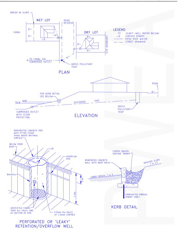
Figure D8.4 **Typical Stormwater Management**
