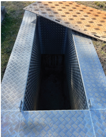
Sleeve in use for a double depth grave
