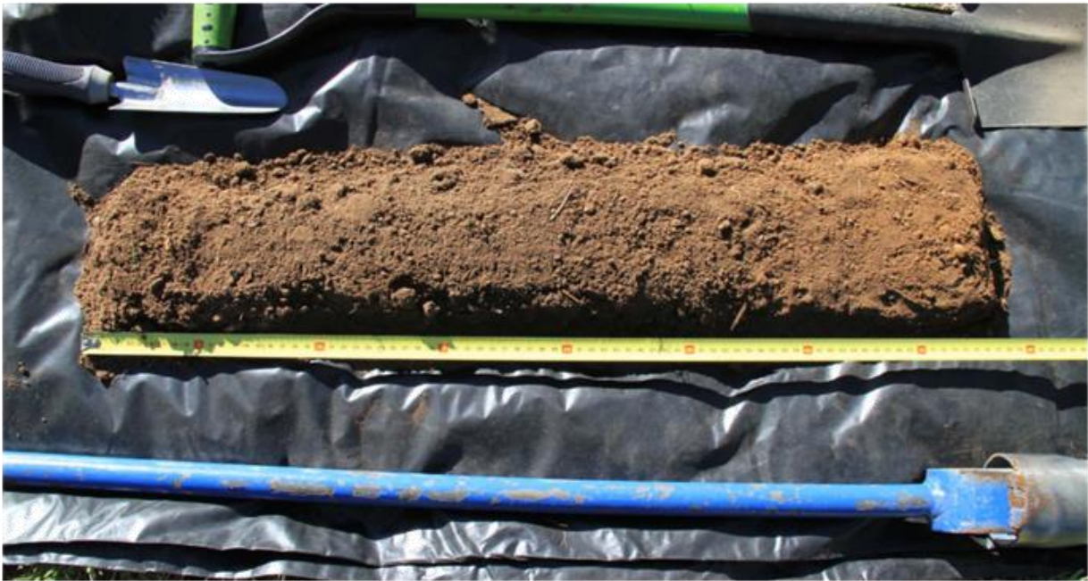
Figure 21. Soil sample taken on site with a hand auger(Photo: Arterra)
