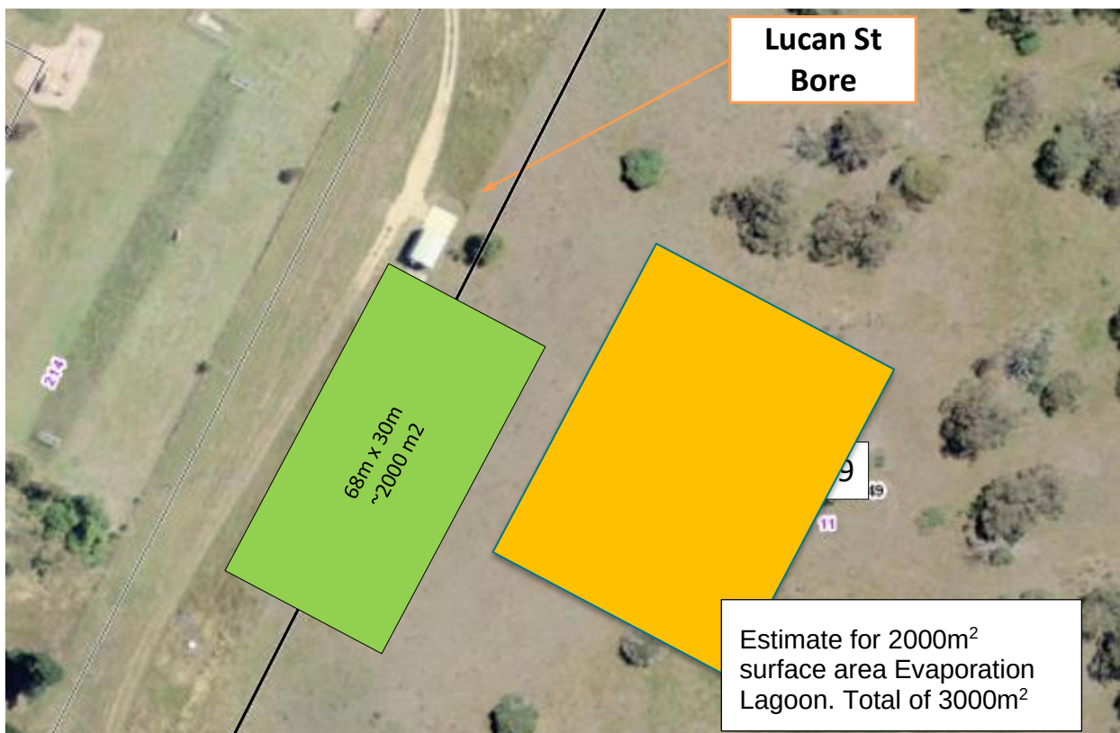
Figure 6-17 High level estimate of a "3 month" evaporation Lagoon
