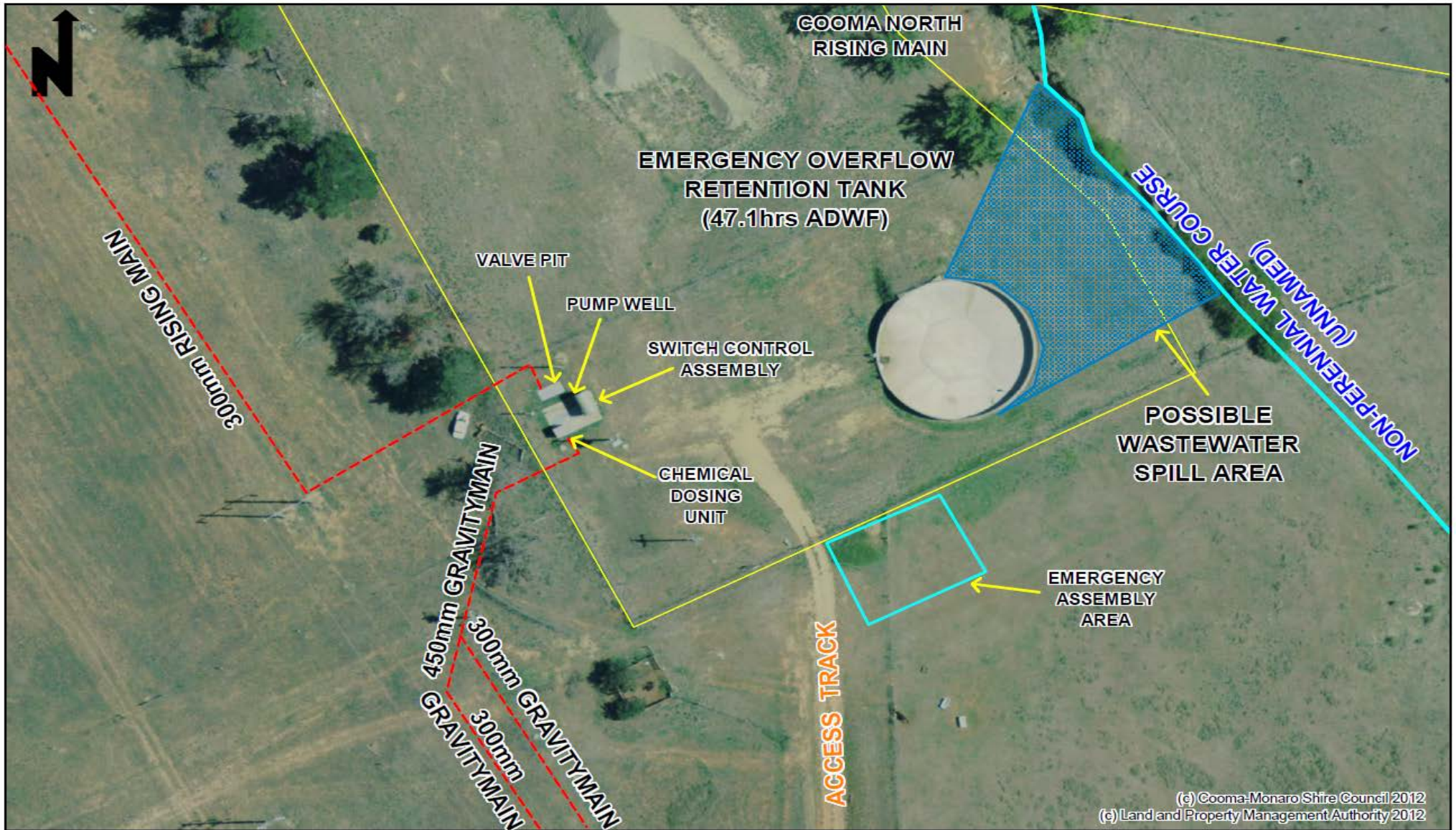
COOMA NORTH WASTEWATER PUMPING STATION - SITE PLAN POLLUTION INCIDENT RESPONSE MANAGEMENT PLAN
