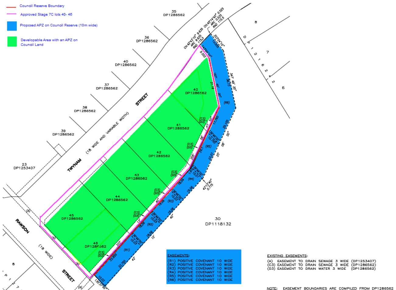
Figure 7: Asset Protection Zone diagram with an APZ on Council Land
